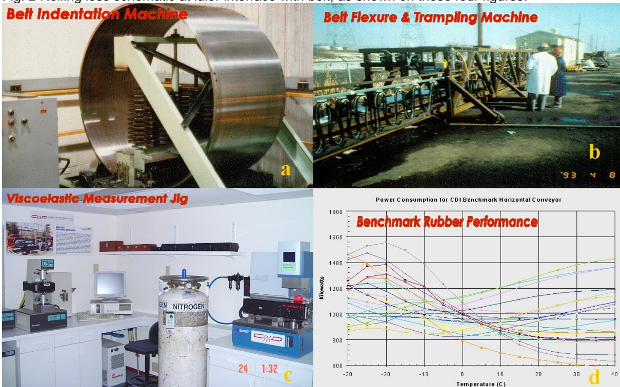
Fig. 3 Belt indentation test machine, belt flexure and trampling test machine, viscoelastic measurement test machine, benchmark rubber performance graph
